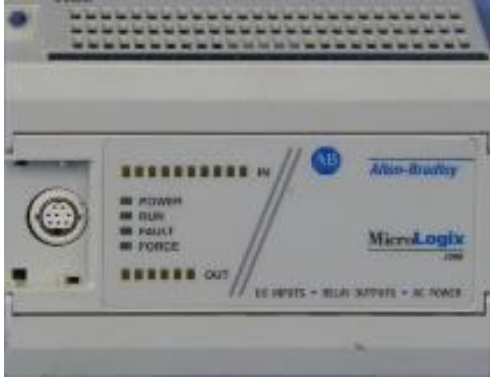
Fixed I/O type of PLC
