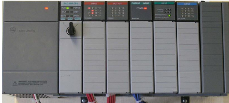
Modular I/O system Mounted in an I/O chassis
